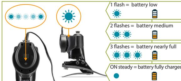
When the IC pod is attached to the foot and being charged, the IC pod LED light will pulsate slowly between ON and OFF and the charging LED on the foot will indicate charging status of the battery by flashing repeatedly – refer to diagrams.
