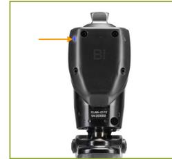
Left side LED on ElanIC indicates current battery charge level and also Bluetooth® status.
