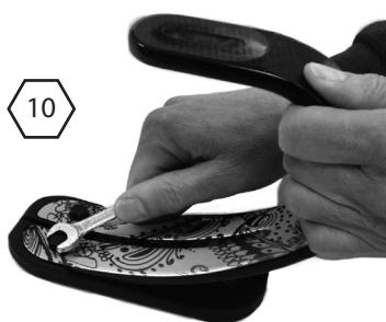
Undo the 2 Heel Spring retaining bolts.
