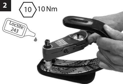
Fit the Toe Spring into the Heel Spring cover and tighten the bolts to 10 Nm.
